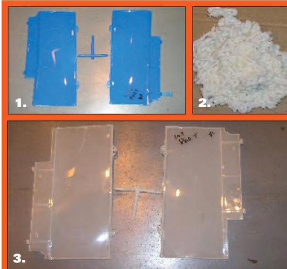
Just 6.5 lbs. of Dyna-Purge cleaned all color from the machine: (1) Last part of 20 run, using blue color; (2) Last of Dyna-Purge compound; (3) First subsequent part using only virgin polypropylene.
