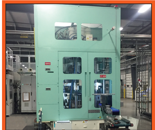
Currier Plastics operates six ISBM machines to produce PET bottles and purges up to five times per week.
