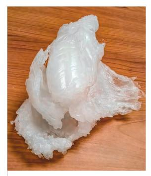
You can avoid clumping or "balling up" in the feedthroat by keeping it cool. This will help solve streaking or specks caused by the hopper or feeding system.
