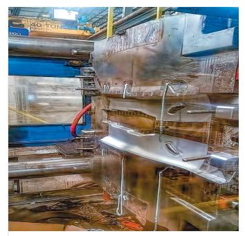
If your hot runners are valve gated and you are experiencing problems with one or more gates, close the other gates and purge the troublesome one(s) separately to increase pressure and turbulence.
